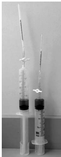
Figure 1 The headspace gas detection tube apparatus prior to (left) and after (right) headspace expulsion through the gas detection tube.
