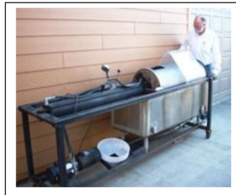
(Above) Jim Schade stands next to his unusual hydraulic horizontal basket press his son designed and helped him to build.
