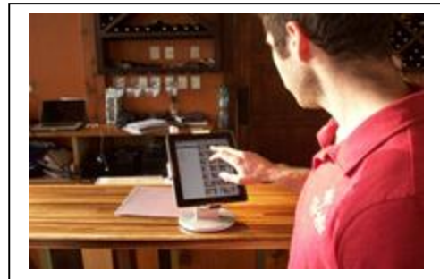
(Above) Will Kimberley uses his I-pad with a free App called “ Square ” to make on-premise sales. Credit cards can be swiped for a 2.75% fee. An I-Phone can also be used for this. Everything uploads via WiFi to the Cloud for data storage. Receipts are sent via e-mail or text messaging. Monthly transactions can be downloaded into a spreadsheet program. 5-15-11
