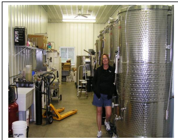
(Above) Gwen Seda (winemaker) standing next to variable capacity tank in their wine cellar. The walls are covered with painted sheet metal and the ceiling is 12' high. 6-9-11
