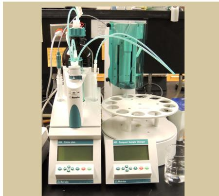
The new autotitrator has given a big boost to everyday chemical analysis efficiency. Lab assistants can simply load samples and within minutes we have a printout with accurate PH and TA measurements.
