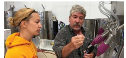
Drew Horton performs an ATP swab measurement for Anne Zwink at Soldier Creek Winery.
