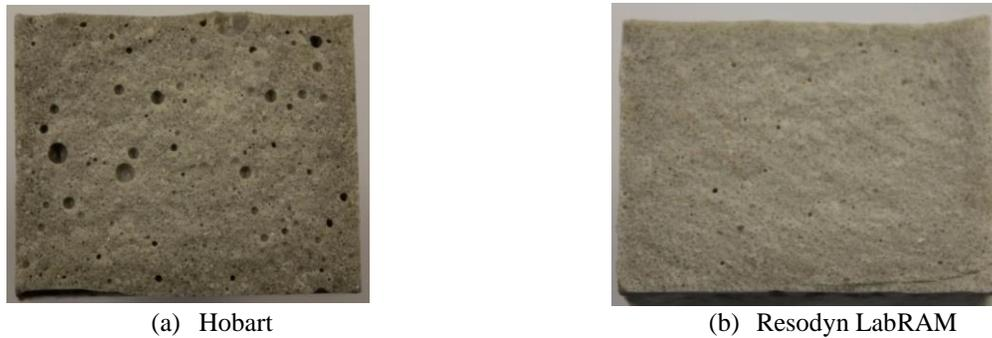
**Figure 6** A visual inspection of the hardened state.
