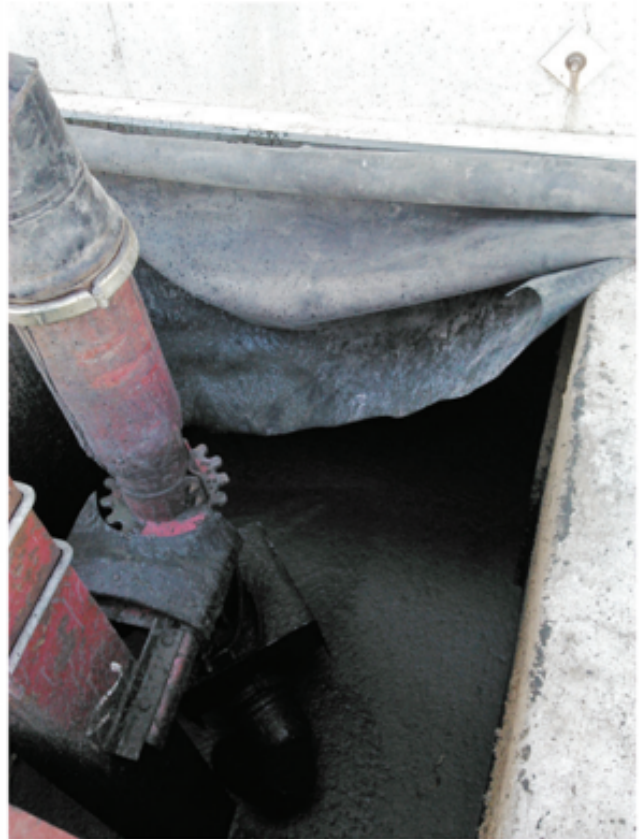
Figure 1: Adding pump out curtains during manure agitation helps limit air exchange of hydrogen sulfide near the applicator.
