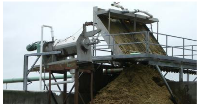
Figure 1. Inclined screen solid-liquid separator.
