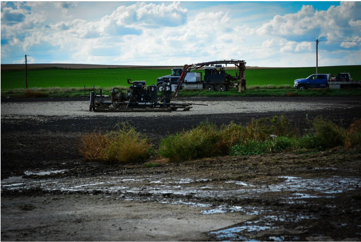
Figure 1. Beginning manure agitation of a dairy lagoon.
