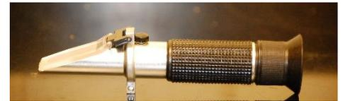
There have been some recent reports of the possibility of using a Brix refractometer to assess passive transfer. The procedure is identical as previously described but the reference values are yet to be unified, acceptable readings fall between 7.8 and 8.4% Brix.
