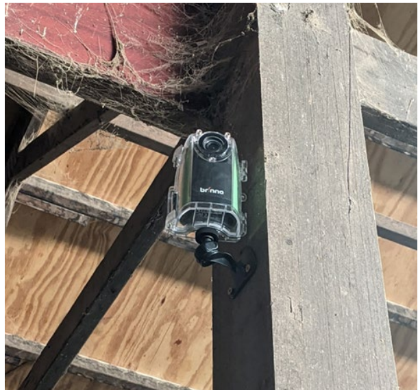
Figure 2. Brinno TLC200 time-lapse camera package with protective case and adjustable swivel wall mount.
