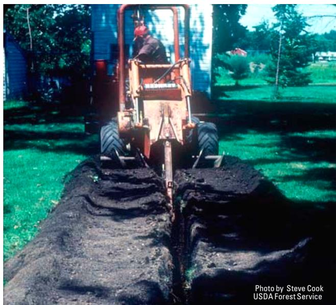
Figure 14. A trenching machine can be used to break root grafts between adjacent oaks of the same species.
