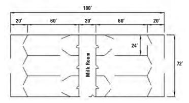
**Example 2.** 2-pen layout to house 60 calves utilizing one auto feeder machine. This allows adequate space for the calves and provides a milk room to house auto feeder and supplies.
