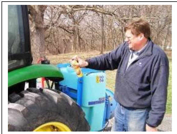
(Above) David Klodd sprays PAM cooking oil on tractor before spraying liquid lime sulfur with the air blast sprayer. Sulfur is very corrosive and easily stains a paint finish. Dave ended up using one 8 oz. $3.49 can of spray to cover the entire tractor.
