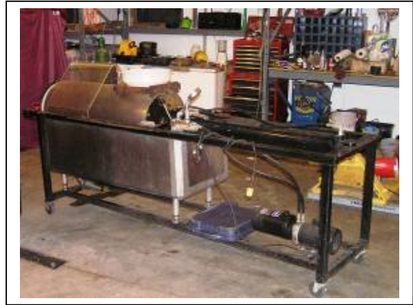
(Above Right) Horizontal hydraulic grape press Jim Schade and his son fabricated themselves. View this in action in the video on their Homepage here: http://www.schadevineyard.com/
