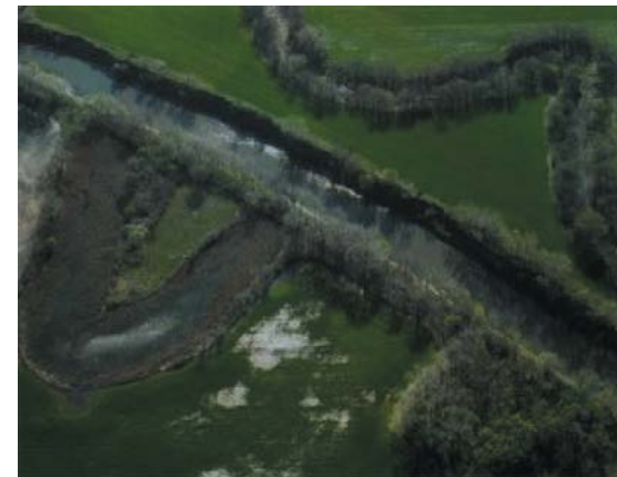
Channelized waterway; original stream bed is still visible.
